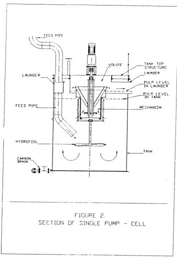
The heart of the mechanism is a low speed rotating impeller. The impeller lifts pulp from inside the cylinder screen and deposits it in the launder above the level of the pulp in the con-
